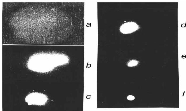
Fig. 3. Photos of beam diameter in the absence of plasma (a) and after beam passing through the plasma for different voltages on electrodes of plasma source: b -  $U = 5$  kV, c -  $U = 6$  kV, d -  $U = 7$  kV, e -  $U = 8$  kV, f -  $U = 9$  kV.
