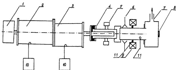
Fig. 1. Scheme of the installation. (1) proton injector; (2) initial stage of accelerator; (3) final stage; (4) plasma gun; (5) gas valve; (6) horn antenna; (7) chamber; (8) luminescent screen; (9) solenoid; (10) RF sources; (11) magnetic field probes.
