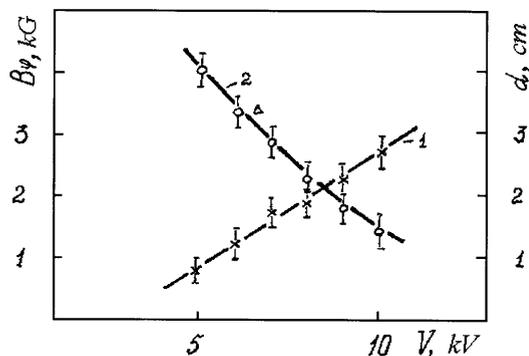
Fig. 2. Dependence of the azimuthal magnetic field  $B_\phi$  (1) and plasma diameter  $d_1$  (2) at the distance of 3 cm from the end of the plasma source upon the electrode voltage.
