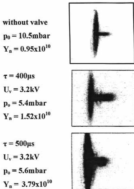
Fig. 3. Soft X-ray pinhole pictures, which were taken with a pinhole camera from discharges performed in the PF-360 facility with the gas puffing, at  $U_0 = 30\text{ kV}$  and  $W_0 = 122\text{ kJ}$ . The figure makes possible to perform a comparison of pictures taken for shots without and with D<sub>2</sub> puffing at different values of a time delay ( $\tau$ ).
