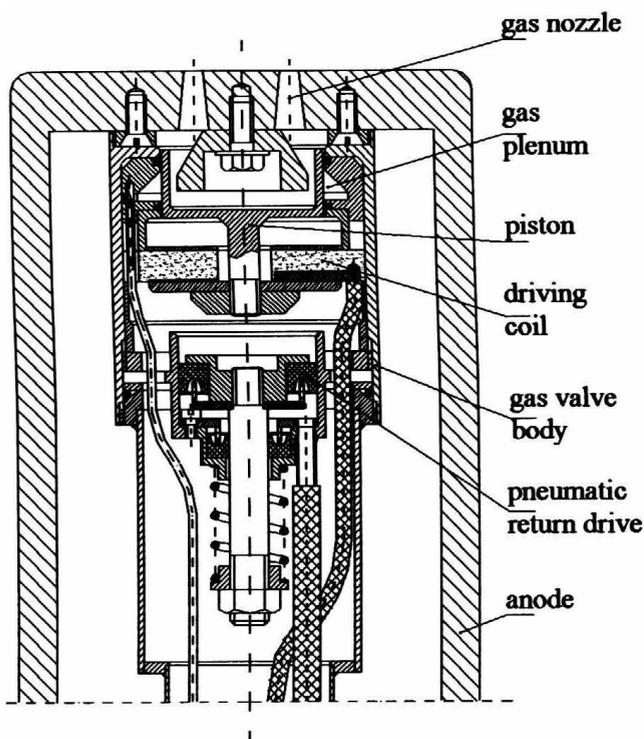
Fig. 1. Assembly of a fast high-pressure gas valve, as designed for gas puffing experiments with the PF-360 facility.
