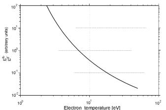
**Fig. 1.** Ratio of the recombination  $(\varepsilon^{/b})$  and bremsstrahlung  $(\varepsilon^{/f})$  emission coefficients as a function of electron temperature.
