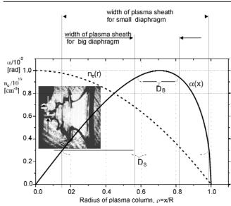
Fig. 6. Influence of the parabolic plasma distribution on laser beam diffraction.
