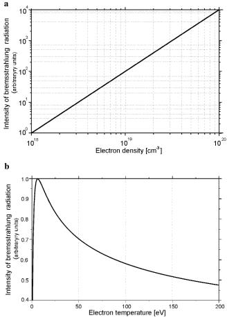
**Fig. 2.** Dependence of the bremsstrahlung radiation on electron density (a), and electron temperature (b).
