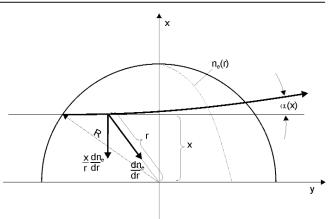
Fig. 4. Illustration of the light ray propagation through in homogeneous plasma.
