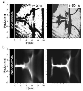
**Fig. 7.** Images of plasma from shadowgraphy (a) and the optical camera (b) for two different moments of the plasma-focus phenomenon.
