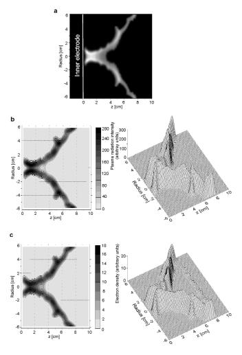
**Fig. 3.** Treatment of the electron density distribution determination: a - the plasma picture, b - the plasma radiation intensity distribution after the Abel transformation, c - the electron density distribution.
