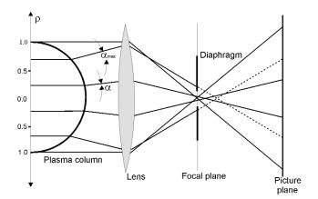
**Fig. 5.** Scheme of the shadowgram registration of axial symmetrical plasma; dashed lines behind the diaphragm denote rays stopped by diaphragm.
