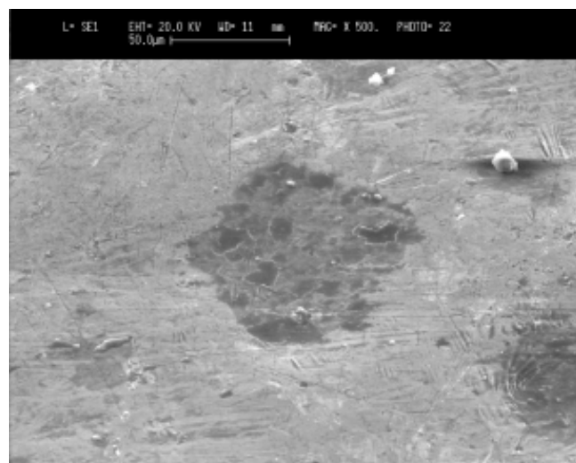
Fig. 8. The electron scanning of the part of the Cu-4mass%Ni alloy sample surface after 3 pulses of the hydrogen plasma actions. One can see the impurities as the dark spots on the surface.
