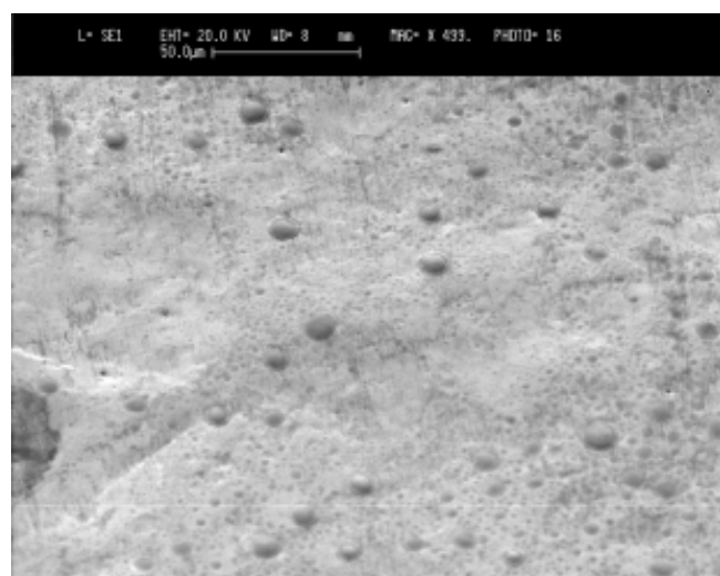
Fig. 4. The electron scanning of the part of 10Cr12Mn20W steel sample surface after 6 pulses of the hydrogen plasma actions. The blisters are visible on the wave like irradiated surface.
