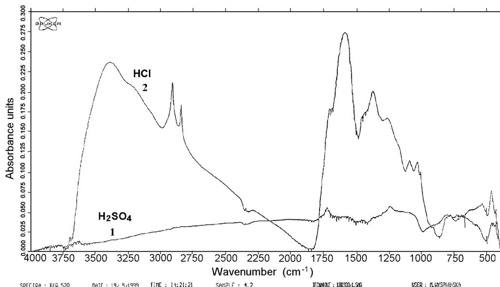
Fig. 6. IR spectrum of Fluka HA eluted with H<sub>2</sub>SO<sub>4</sub> (1) or HCl (2).
