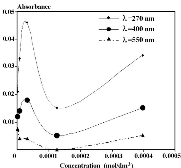
Fig. 5. UV absorbance of eluates (diluted 1:50) after HA washing with  $\text{H}_2\text{SO}_4$  of different concentrations.
