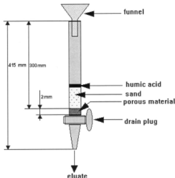
Fig. 1. The separation column of  $\varnothing=13$  mm.
