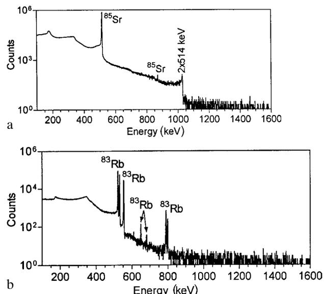
**Fig. 2.** a – Gamma spectrum of the separated <sup>85</sup>Sr tracer, measured with a low background shielded germanium detector. Beside the main <sup>85</sup>Sr photopeak at 513.99 keV (98.3%), the summing effect peak at 1028 keV and a weak line at 868 keV (0.012%) are visible. Counting time 1 h. b – Gamma spectrum of the separated <sup>83</sup>Rb tracer, measured with a low background shielded germanium detector. Counting time 5.2 h.
