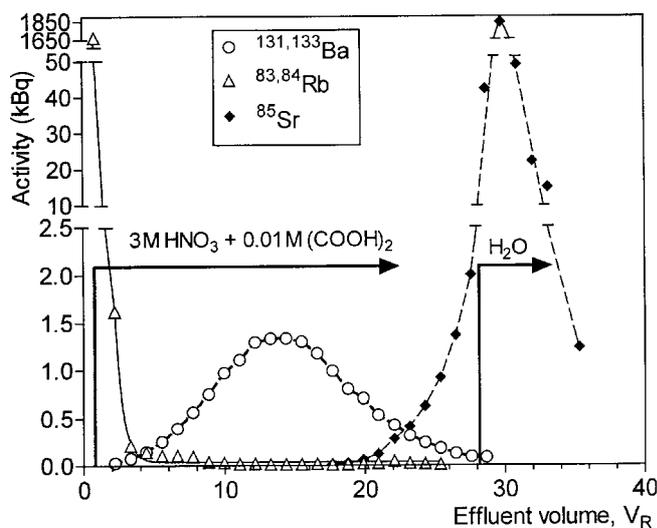
**Fig. 1.** Elution of Rb<sup>+</sup>, Ba<sup>2+</sup> and Sr<sup>2+</sup> ions on the Sr-Resin column. The units on the horizontal axis are the resin volumes ( $V_R = 2.9$  cm<sup>3</sup>) of the column. Flow-rate  $0.8 \pm 0.1$  cm<sup>3</sup> per minute (for the small Sr-Resin column: flow-rate is about 0.1 cm<sup>3</sup> per minute and  $V_R = 0.21$  cm<sup>3</sup>).
