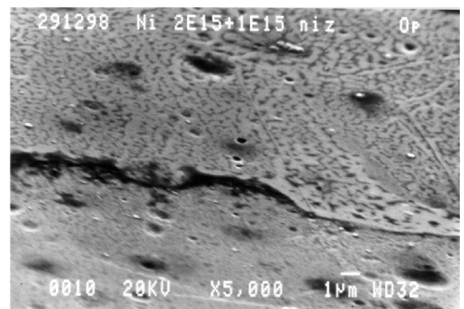
Fig. 2. The surface structure of polycrystalline Ni previously irradiated with 305 MeV ^{86}\text{Kr} ions up to the fluence F \cdot t = 2 \times 10^{15} ions/cm ^2 and then irradiated with 245 MeV ^{86}\text{Kr} ions up to the fluence of F \cdot t = 1 \times 10^{15} ions/cm ^2 (the upper part was covered by mask). One can see a step on the boundary between single- and double-irradiated regions.
