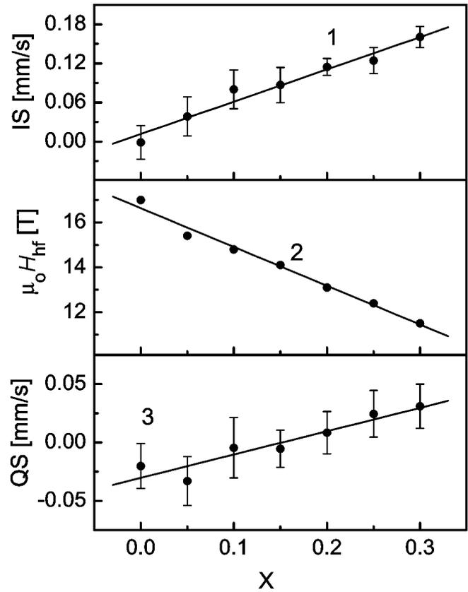
**Fig. 2.** Average hyperfine interaction parameters of the Dy(Mn<sub>0.4-x</sub>Al<sub>x</sub>Fe<sub>0.6</sub>)<sub>2</sub> series (77 K): 1 – the isomer shift IS in relation to Fe-metal, 300 K; 2 – the magnetic hyperfine field  $\mu_0 H_{\text{hf}}$ ; 3 – the quadrupole interaction parameter QS.
