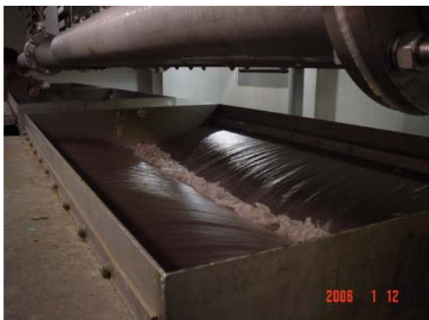
Fig. 1. Industrial e-beam plant for textile dyeing wastewater in Daegu, Korea.
