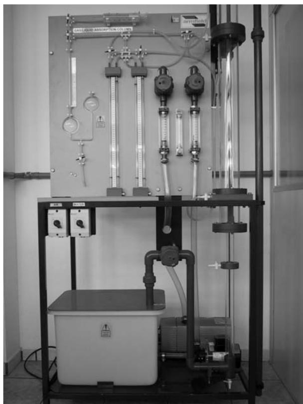
**Fig. 4.** Laboratory gas absorption column for multiphase system analyses.
