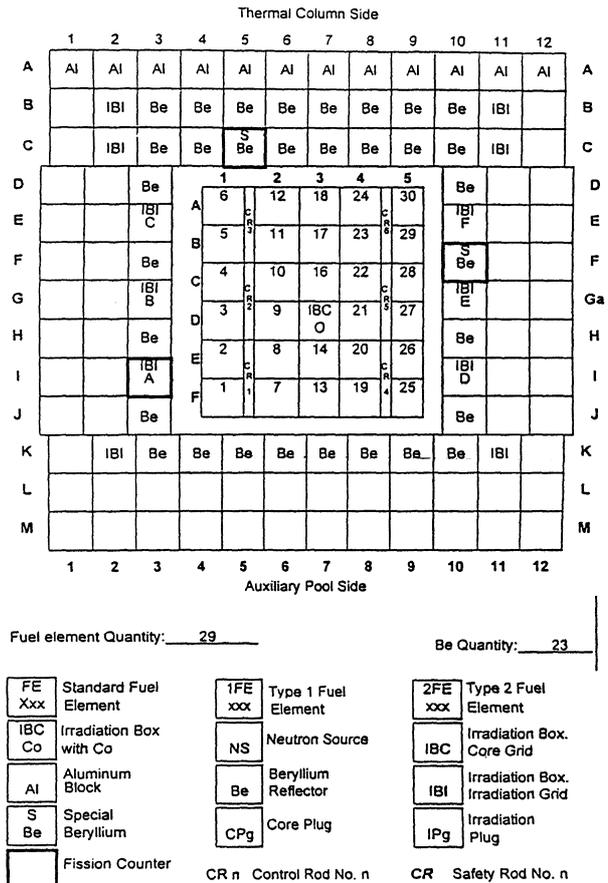
**Fig. 2.** First core configuration: FE – 404.7 gm U-235; 1FE – 148.2 gm U-235; 2FE – 209.0 gm U-235.
