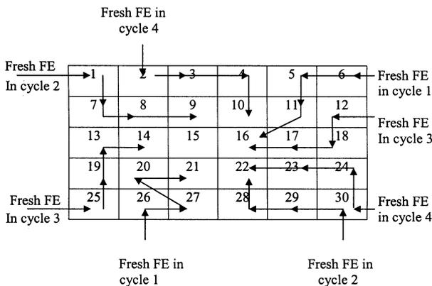
**Fig. 4.** First shuffling scheme in periodic 4 cycle.
