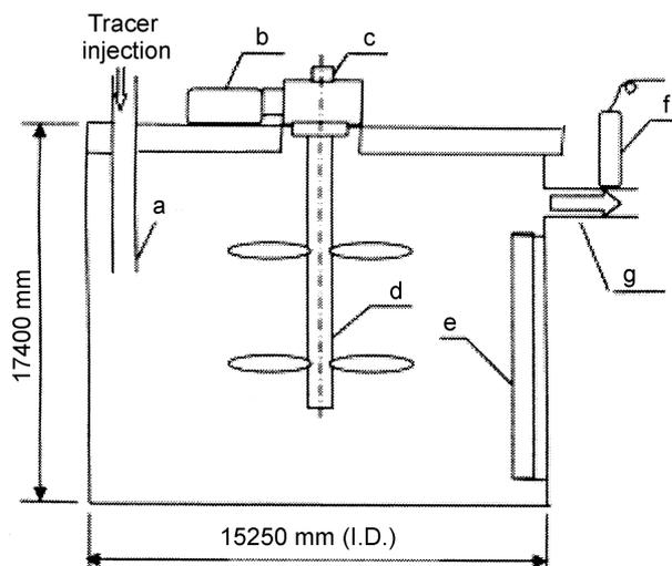
**Fig. 2.** Schematic diagram of tank: a – inlet pipe; b – motor and drive mechanism; c – sparge sleeve; d – shaft with impellers; e – baffle; f – detector; g – outlet stream.
