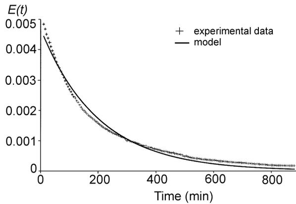
Fig. 6. Perfect mixer model fit of experimental data.
