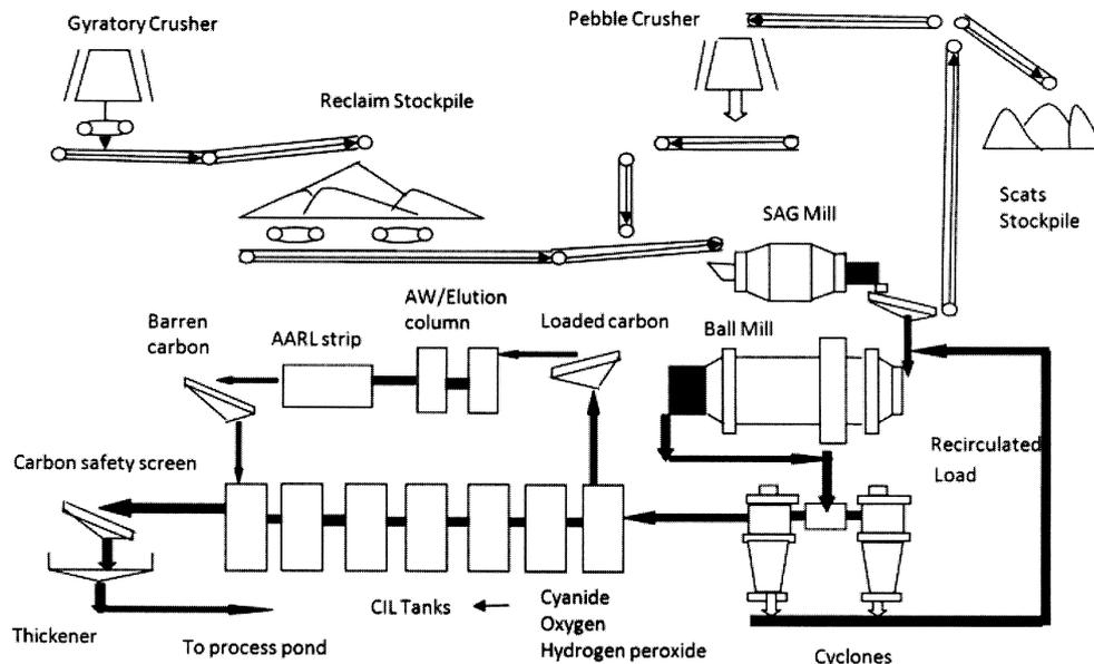
**Fig. 1.** Flow diagram of gold ore processing at Damang Mine.
