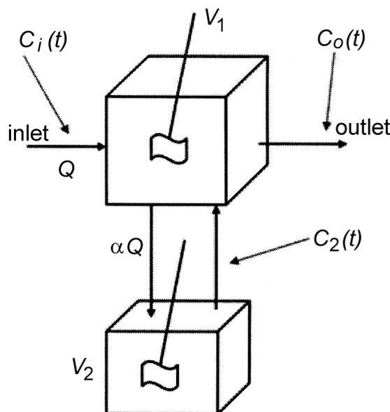
Fig. 5. Schematic diagram of mixing cells with exchange model.
