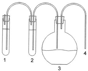
Fig. 5. Vacuum transfer system used in the assay no. 5.
