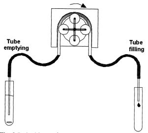
Fig. 6. Peristaltic transfer system.
