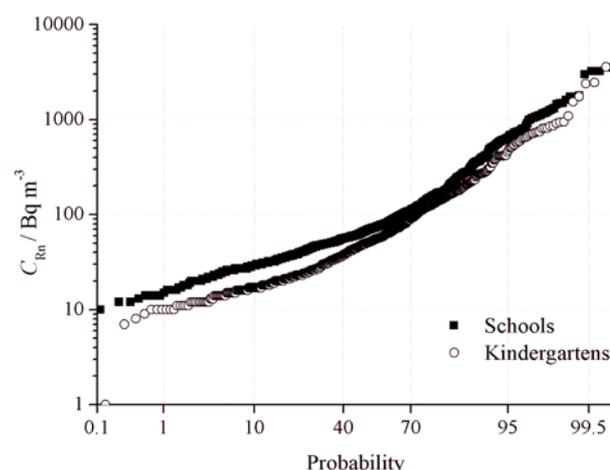
**Fig. 1.** Lognormal plots of radon concentrations in 730 kindergartens and 890 schools, obtained in wintertime with alpha scintillation cells in rooms closed overnight prior to measurement.
