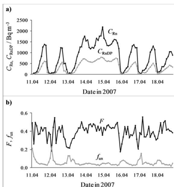
**Fig. 3.** Results of a continuous measurement of concentrations ( $C_{Rn}$  and  $C_{RnDP}$ , respectively),  $F$  between Rn and RnDP and unattached fraction ( $f_{unatt}$ ) of RnDP.
