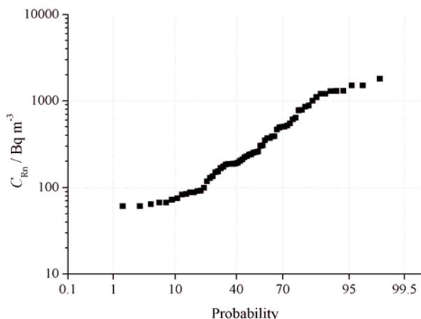
**Fig. 6.** Lognormal plot of radon concentrations obtained with track etch detectors in 64 rooms of 24 public buildings.
