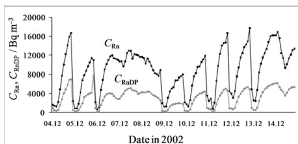
**Fig. 4.** Time series of concentrations of Rn and RnDP obtained with continuous measurement in a hospital room with high radon level.
