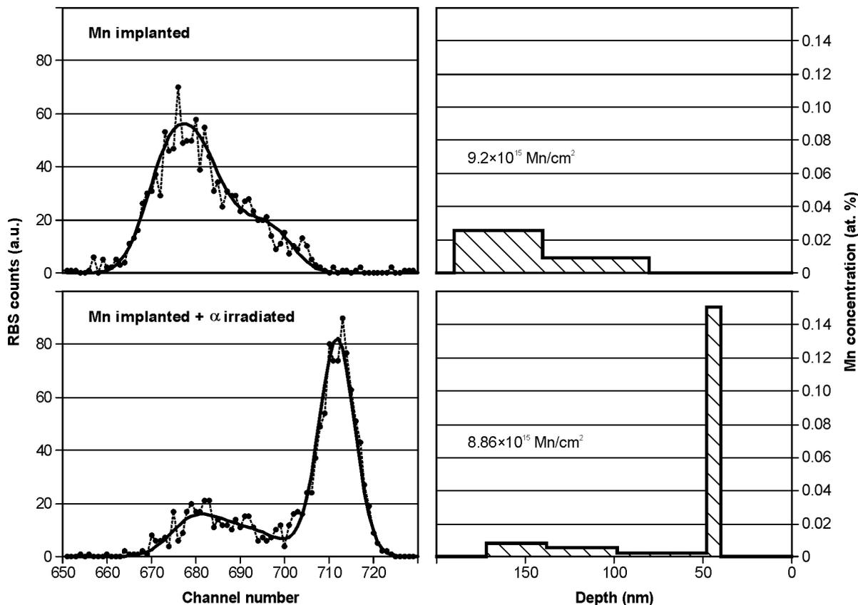
**Fig. 3.** Results of SIMNRA simulations of Mn profiles before and after <sup>4</sup>He<sup>+</sup>-irradiation. Left: RBS spectra. Right: Mn depth profiles (please note the depth scale direction).
