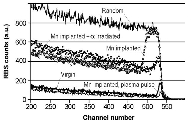
**Fig. 1.** Random and channeled RBS spectra corresponding to a virgin silicon sample and channeled spectra of Mn-implanted/implanted and  $^4\text{He}^+$ -irradiated/hydrogen-plasma-pulse-treated samples.
