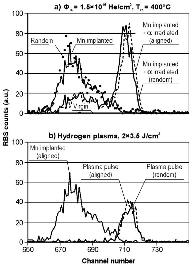
**Fig. 2.** Random and channeled RBS spectra illustrating manganese evolution after (a) <sup>4</sup>He<sup>+</sup>-irradiation and (b) hydrogen-pulse-plasma treatment.
