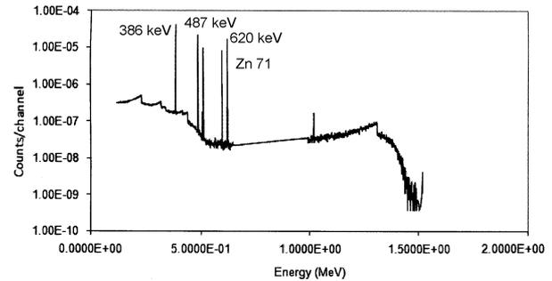
**Fig. 2b.** A sample of learning data containing  $^{71}\text{Zn}$ .
