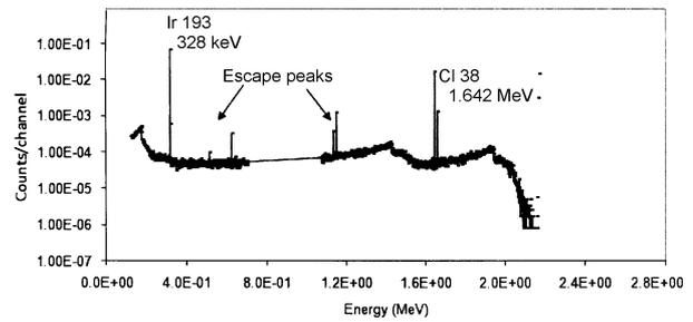
**Fig. 2a.** A sample of learning data containing  $^{38}\text{Cl}$  and  $^{193}\text{Ir}$ .
