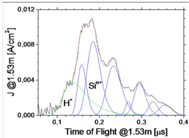
Fig. 4. The deconvolution of the ICS-TOF spectrum.
