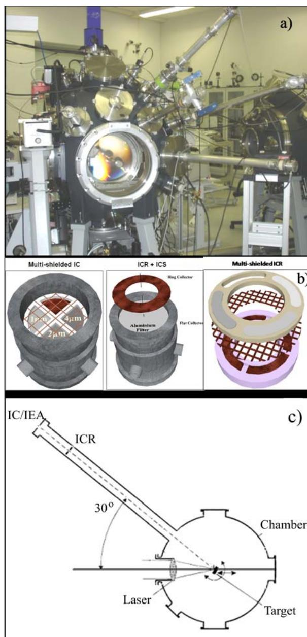
**Fig. 1.** (a) Photo of the interaction chamber at PALS; (b) the three different IC configurations; (c) a sketch of the experimental setup.
