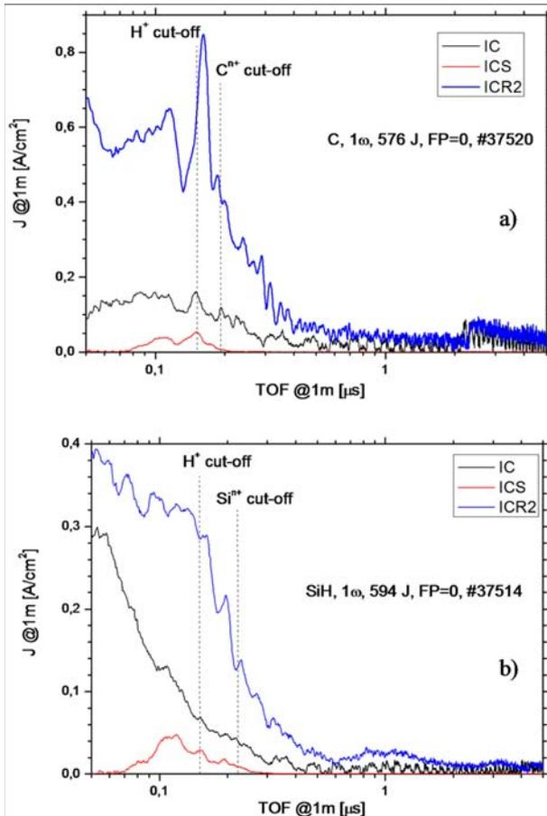
**Fig. 2.** Typical TOF spectra registered on different IC's for (a) the graphite target, and (b) for the hydrogenated annealed silicon target.
