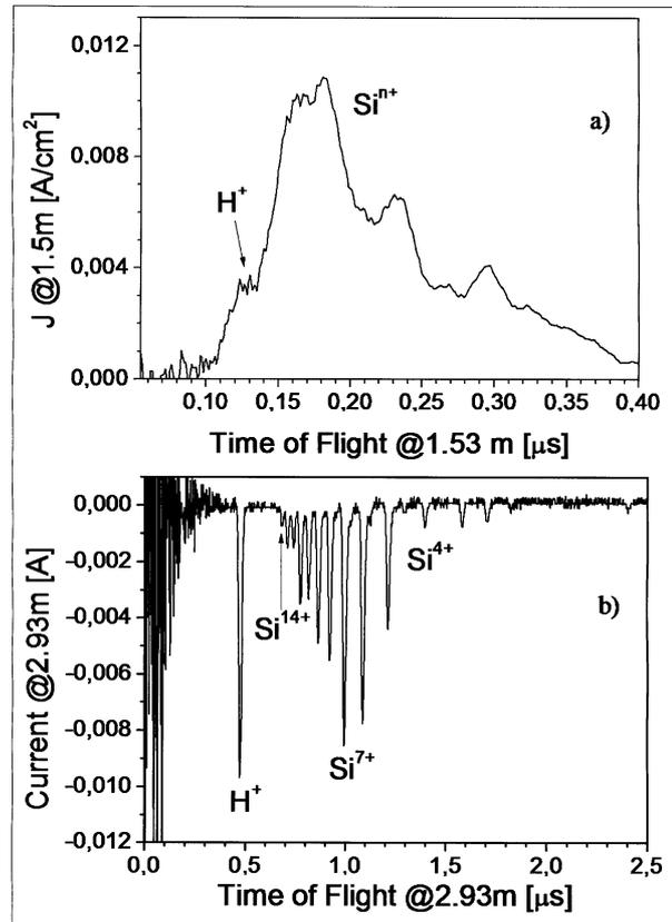
**Fig. 3.** (a) The shielded ion collector (ICS) TOF spectrum; (b) the IEA spectrum for a hydrogenated annealed silicon target.
