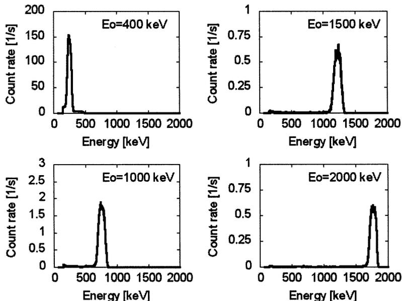
**Fig. 5.** Energy spectra of helium ions scattered on a gold foil of  $100 \mu\text{g}/\text{cm}^2$ , recorded using the diamond detector.
