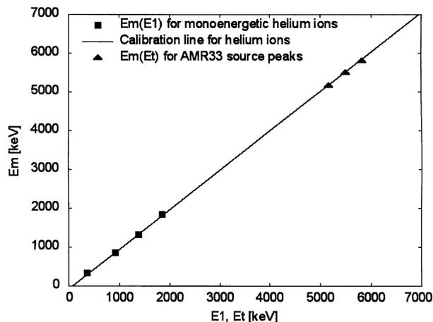
**Fig. 6.** Measured values of  $E_m$  vs. the reference (beam  $E_1$  or source  $E_t$ )  $\alpha$  energy.
