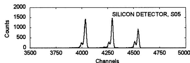
**Fig. 3.** Spectra of the AMR33 source recorded with the diamond and silicon detectors.
