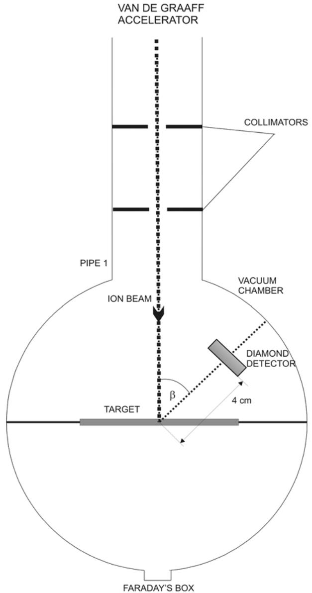
**Fig. 4.** Geometry of the detection of the backscattered ions.
