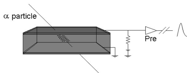
**Fig. 1.** Principle of  $\alpha$  detection by a semiconductor detector.
