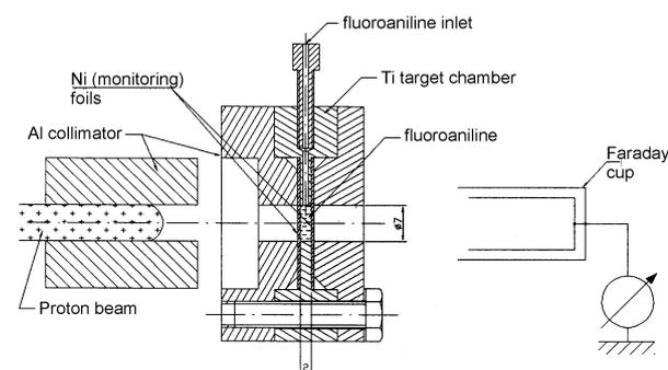
**Fig. 1.** Scheme of the irradiating arrangement. The 25 MeV proton beam passes through the monitoring Ni foil and then through the fluoroaniline sample and the second monitoring Ni foil, and it is stopped in the Faraday cup.
