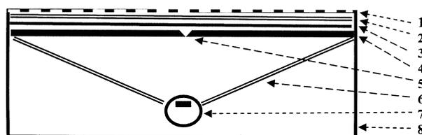
**Fig. 2.** Layout of the scintillation probe. 1 – protection grid; 2 – three layers of aluminized foil; 3 – ZnS(Ag) phosphor on a thin plastic foil; 4 – plastic scintillator  $250 \times 125 \times 1$  mm<sup>3</sup>; 5 – intersection of plastic scintillator; 6 – light reflector; 7 – side window PMT; 8 – light tight housing.
