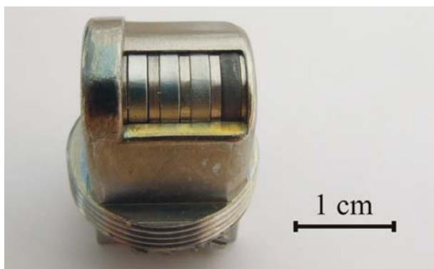
Fig. 1. Picture of the modified Cherenkov-type measuring head for fast electron studies.
