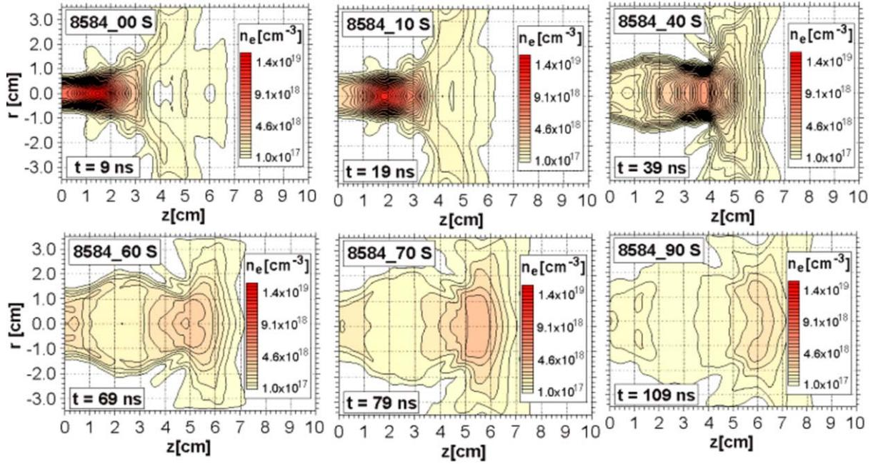
**Fig. 9.** Shot 8584 ( $D_2, p_0 = 2.4$  mbar,  $U_0 = 27$  kV,  $Y_n = 4.2 \times 10^{11}$ ). Equidensity contours reconstructed from interferograms taken at different moments after the minimum of  $dI/dt$ .
