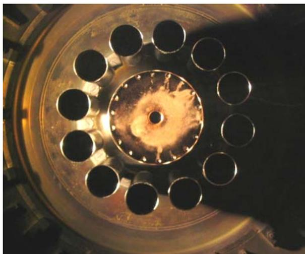
**Fig. 2.** View of the PF-1000 electrodes.
