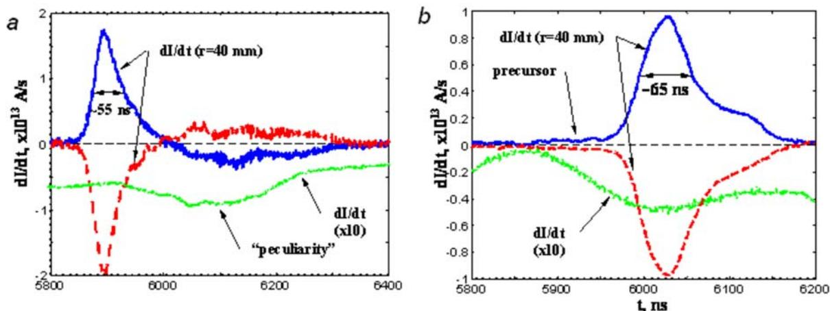
Fig. 6. Results of measurement of the azimuthal magnetic field during two discharges: a – shot 8479 ( $D_2, p_0 = 2.66$  mbar,  $U_0 = 23$  kV,  $Y_n = 1.0 \times 10^{11}$ ), and b – shot 8466 ( $D_2, p_0 = 2.66$  mbar,  $U_0 = 24$  kV,  $Y_n = 1.5 \times 10^8$ ).
