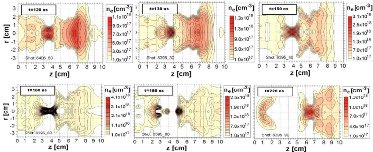
**Fig. 11.** Shot 8406 ( $D_2, p_0 = 2.4$  mbar,  $U_0 = 24$  kV,  $Y_n = 9.0 \times 10^{10}$ ). Equidensity contours reconstructed from interferograms taken at different moments after the minimum of  $dI/dt$ .
