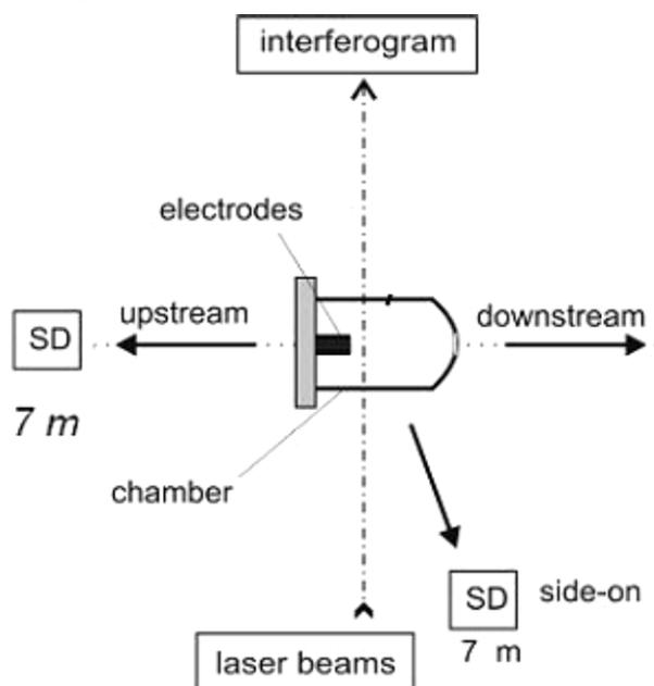
Fig. 5. The arrangement of neutron probes.
