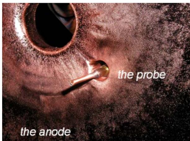
Fig. 4. Setup of the absolute calibrated magnetic probe (ACMP).
