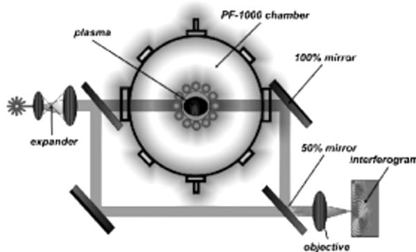
**Fig. 3.** Mach-Zehnder interferometer setup for PF-1000U [7].
