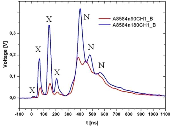
**Fig. 10.** Shot 8584 ( $D_2, p_0 = 2.4$  mbar,  $U_0 = 27$  kV,  $Y_n = 4.2 \times 10^{11}$ ). Four hard X-ray (X) and neutron (N) pulses recorded by PMT probes side-on (A8584n90CH1\_B) and upstream (A8584n180CH1\_B).
