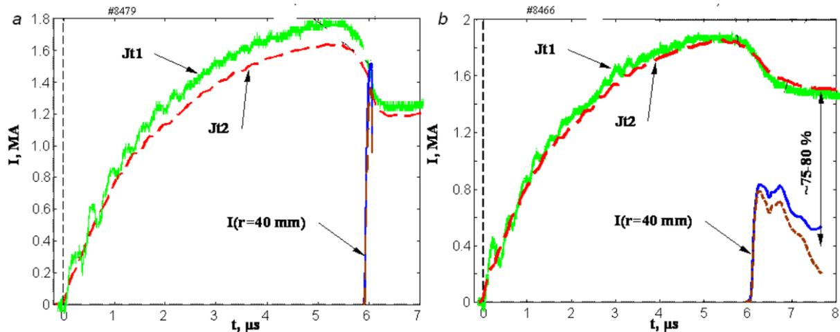
**Fig. 7.** Currents measured by means of the Rogowski coil (Jt1), a single-loop (Jt2) and a probe located at  $r = 40$  mm, a – shot 8479 ( $D_2, p_0 = 2.66$  mbar,  $U_0 = 23$  kV,  $Y_n = 1.0 \times 10^{11}$ ), b – shot 8466 ( $D_2, p_0 = 2.66$  mbar,  $U_0 = 24$  kV,  $Y_n = 1.5 \times 10^8$ ).
