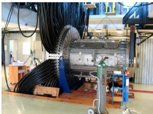
**Fig. 1.** View of the PF-1000 vacuum chamber, collector and HV cables.
