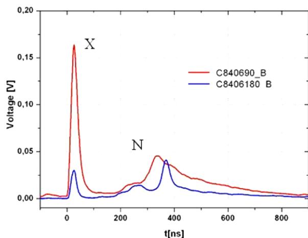
**Fig. 12.** Shot 8406 ( $D_2$ ,  $p_0 = 2.4$  mbar,  $U_0 = 24$  kV,  $Y_n = 9.0 \times 10^{10}$ ). Hard X-ray (X) and neutron (N) pulses recorded by PMT probes side-on (C8406n90\_B) and upstream (C8406n180\_B).
