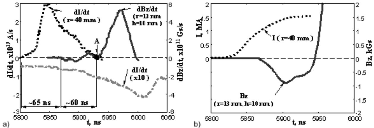
**Fig. 6.** Results of measurements of the azimuthal and axial magnetic field components on the PF-1000 facility: (a) derivative of the total current,  $dI/dt$ , the current derivative, measured by the azimuthal probe at radius 40 mm,  $dI/dt$  ( $r = 40$  mm), and derivative of induction of the axial magnetic field,  $dBz/dt$ , and (b) current within radius 40 mm,  $I$ , and induction of the axial magnetic field,  $Bz$ .
