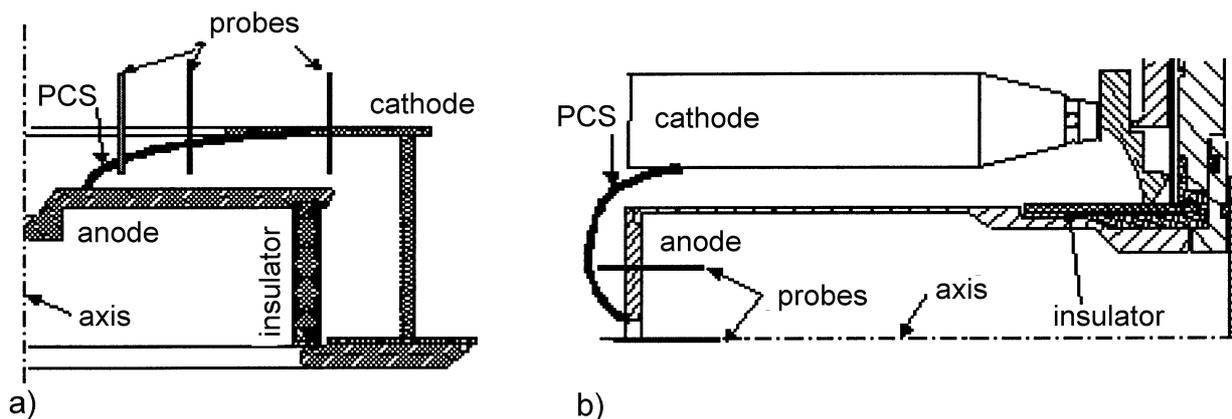
**Fig. 1.** Arrangement of magnetic probes in the (a) PF-3 and (b) PF-1000 facilities. The probes are installed at radii of 460, 260, 160 mm (PF-3), and of 40 and 13 mm (PF-1000).
