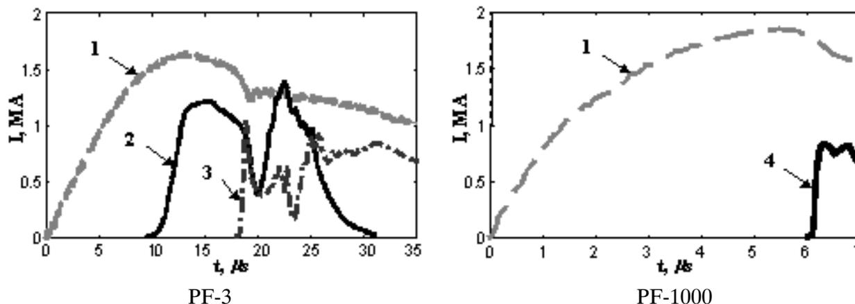
**Fig. 3.** Current oscillograms in nonoptimal discharges: total discharge current (1) and currents measured at distances of 46 cm (2), 16 cm (3) and 4 cm (4) from the axis.
