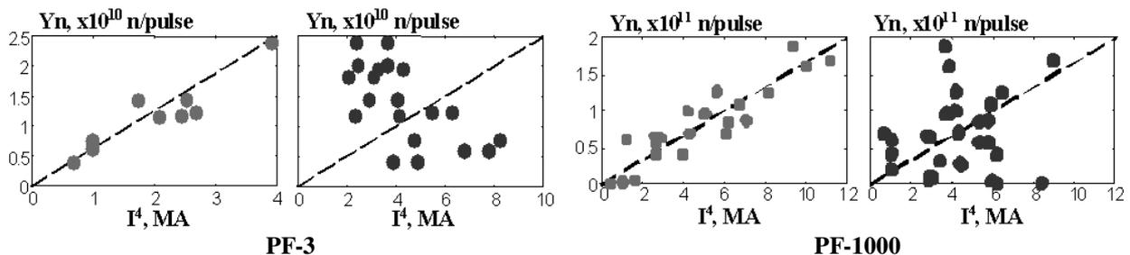
Fig. 5. Neutron yield  $Y_n$  as a function of the current measured by magnetic probes (on the left) and the total current at the instant of neutron generation (on the right). The dashed line shows the dependence  $Y_n \sim I^4$ .
