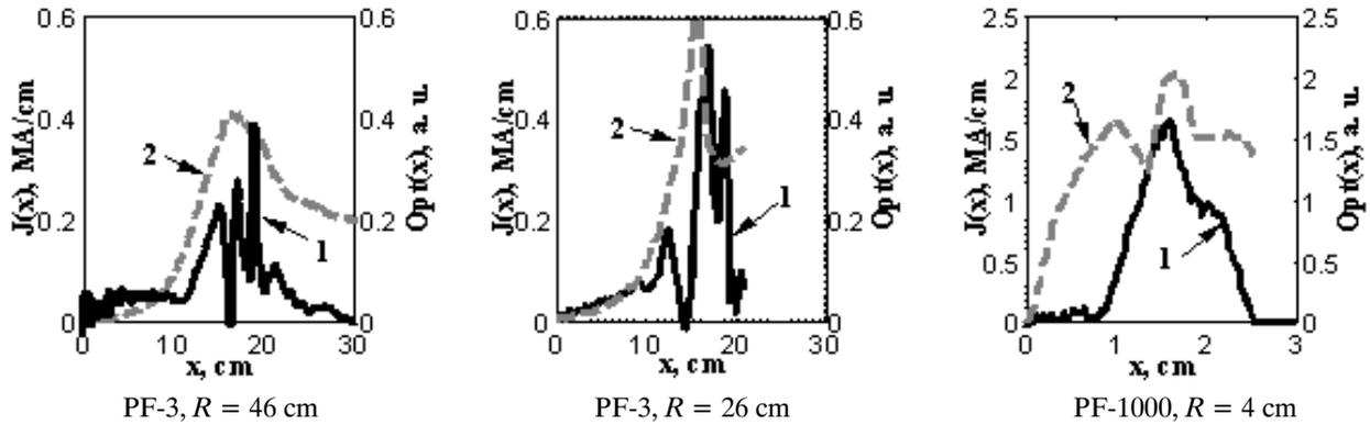
Fig. 4. Profiles of the (1) current density and (2) plasma glow across the PCS in different discharge stages.
