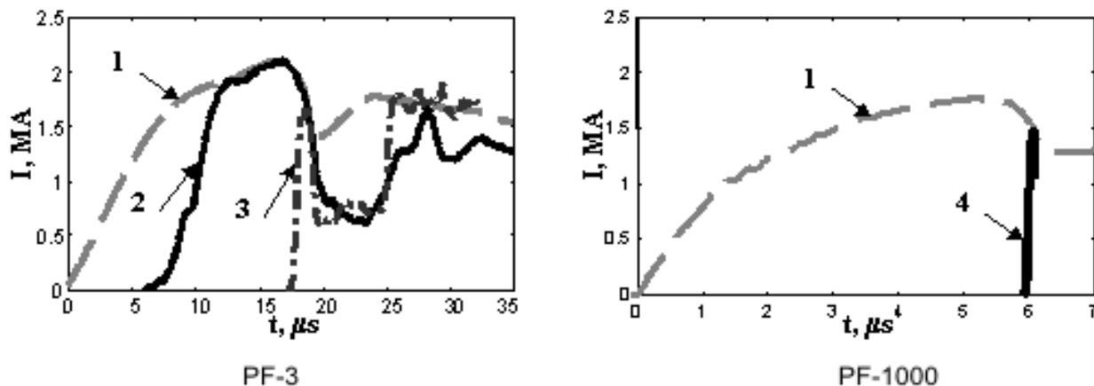
**Fig. 2.** Current oscillograms in optimal discharges: total discharge current (1) and currents measured at distances of 46 cm (2), 16 cm (3) and 4 cm (4) from the axis.
