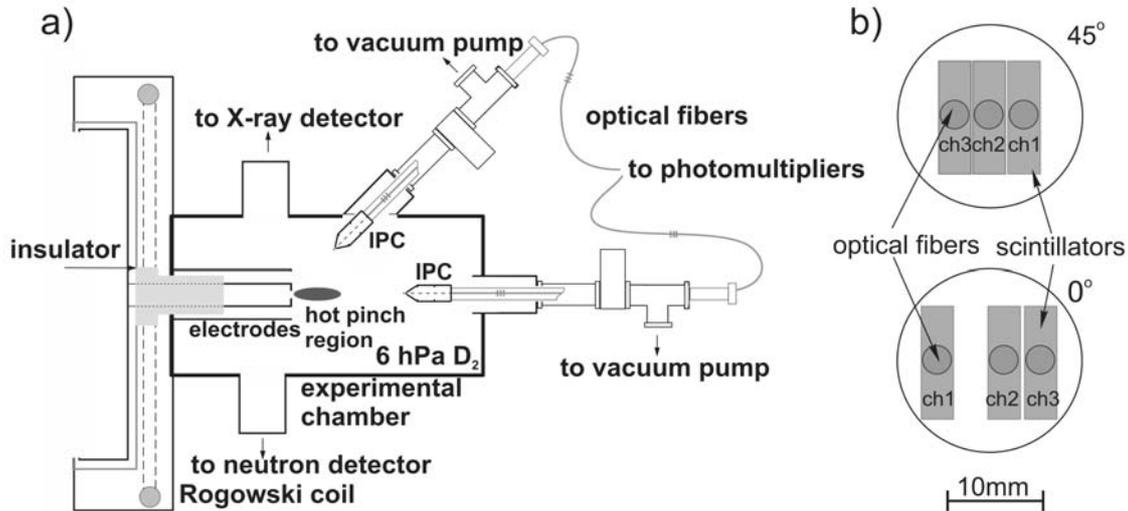
**Fig. 1.** Scheme of the PF-360 experiment (not to scale) which shows positions of ion pinhole cameras (a), and scheme of the scintillation detectors arrangement inside the camera placed at the angle of  $45^\circ$  to the axis (b, top) and along the axis (b, bottom).
