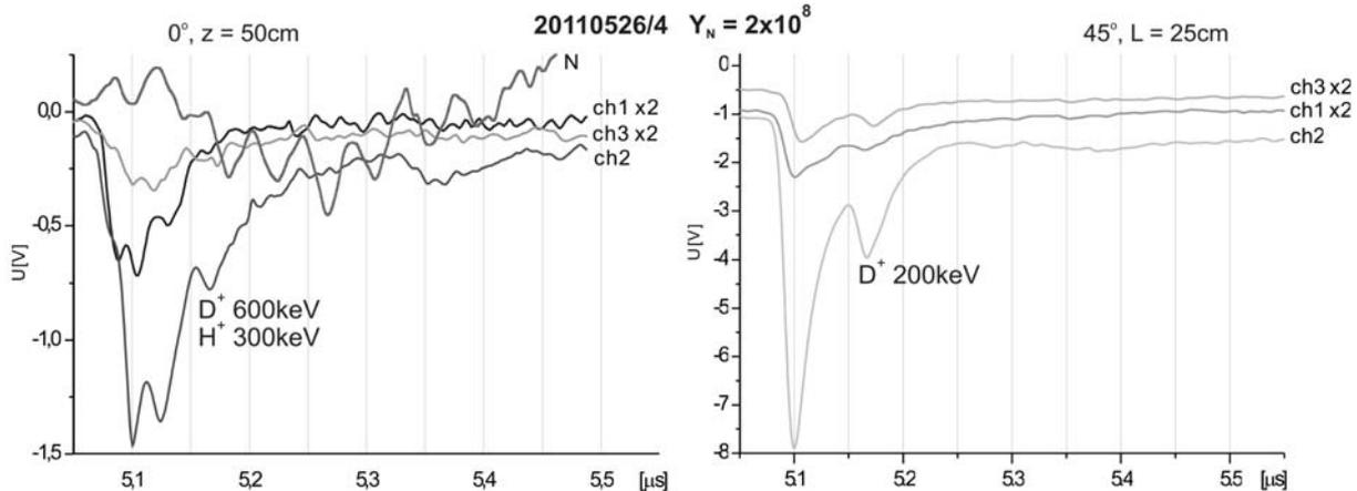
**Fig. 5.** X-ray and ion signals recorded with the IPC placed at  $0^\circ$  and a distance 50 cm (left) and these from the IPC placed at  $45^\circ$  and a distance of 25 cm (right). For a comparison there are also shown signals from a neutron probe (N) or a Rogowski coil (I).
