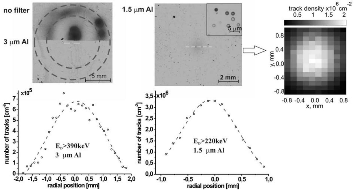
**Fig. 3.** Ion images, density profiles (obtained with different absorption filters) and a track-density map, as recorded with the IPC placed at a distance of 80 cm (left) or 100 cm (right) from electrodes outlets.
