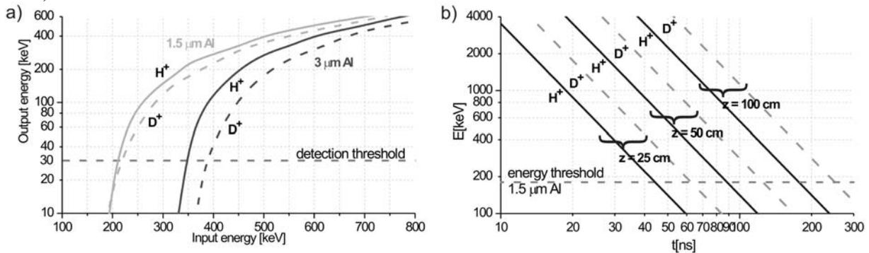
**Fig. 2.** Energy of protons and deuterons after their penetration through an Al-filter of different thickness (a), and TOF of the measured ions over different distances (b).
