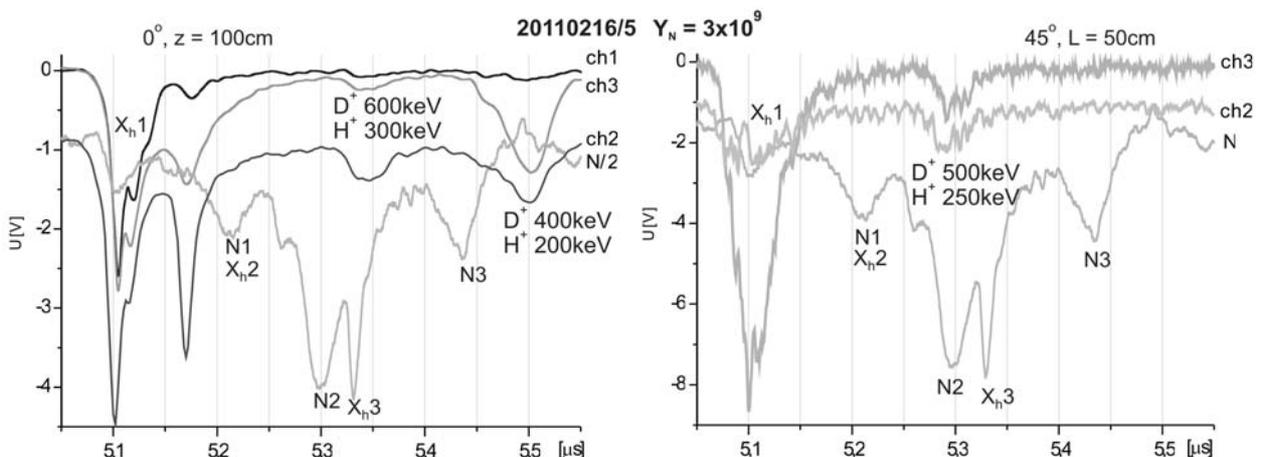
**Fig. 4.** X-ray and ion signals recorded with the IPC placed at  $0^\circ$  and a distance of 100 cm (left) and these from the IPC placed at  $45^\circ$  and a distance of 50 cm (right). Signals recorded by a neutron probe (N) were used for a reference.
