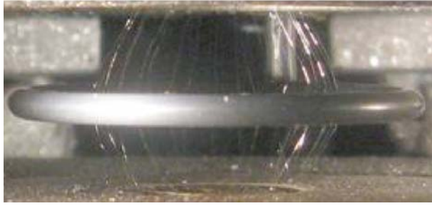
Fig. 4. Electrostatically shaped quasi-spherical wire array with the ring intermediate electrode.
