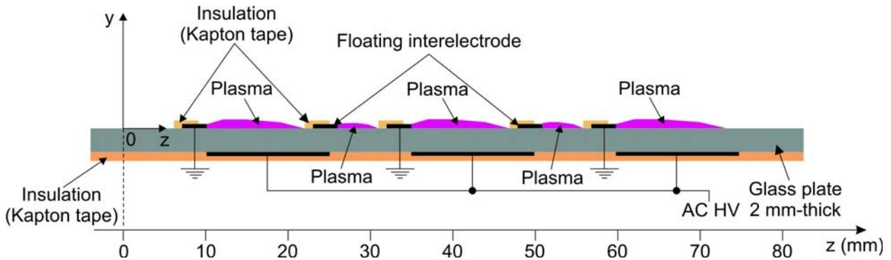
**Fig. 1.** Schematic side view of the multi-DBD actuator with floating inter-electrodes developed for airflow generation investigations.
