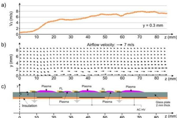
**Fig. 5.** Time-averaged horizontal flow velocity profile taken 0.3 mm above the dielectric surface (a) and the flow velocity vector field (b) of the airflow generated by the multi-DBD actuator (c). The applied sine-wave voltage was  $32 \text{ kV}_{pp}$ , the frequency – 1.5 kHz. FL – floating inter-electrode.
