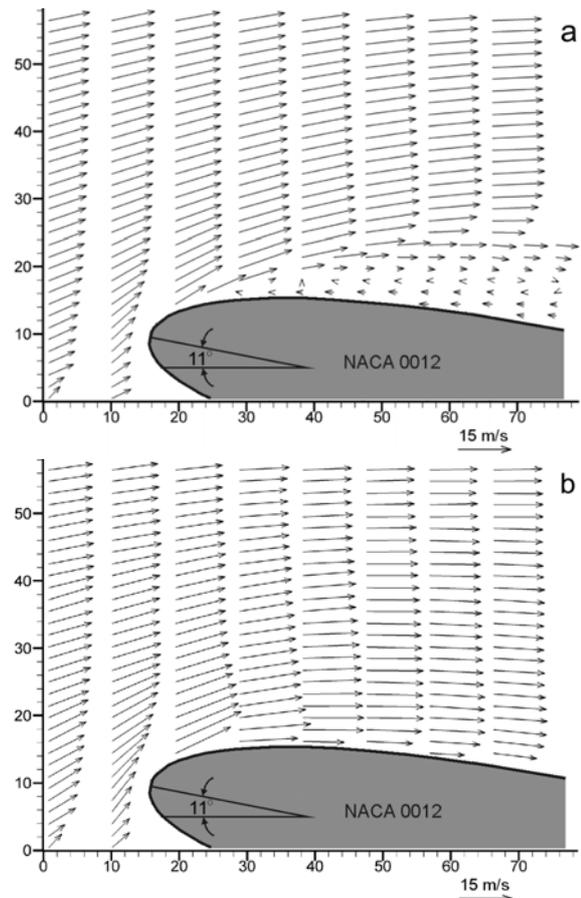
**Fig. 6.** Time-averaged flow velocity vector field of the airflow around NACA0012 airfoil model for the leading edge flow separation control experiment with the multi-DBD actuator turned off (a) and turned on (b). The main flow velocity was 15 m/s and the angle of attack was 11 degrees. The applied sine-wave voltage was  $15 \text{ kV}_{pp}$ , and frequency 1.5 kHz.
