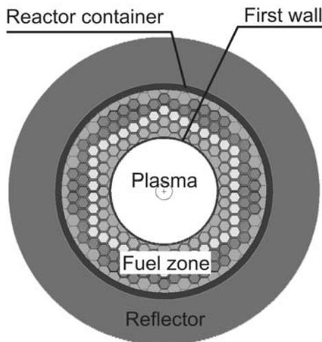
Fig. 1. Hybrid reactor cross section.
