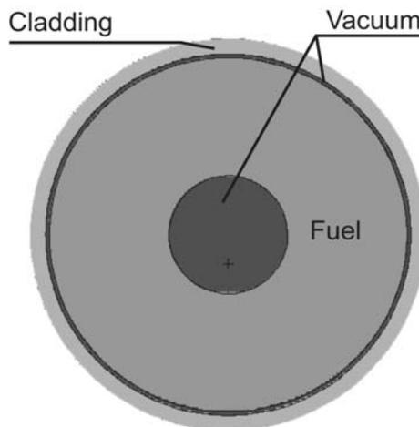
Fig. 3. Fuel rod cross section.
