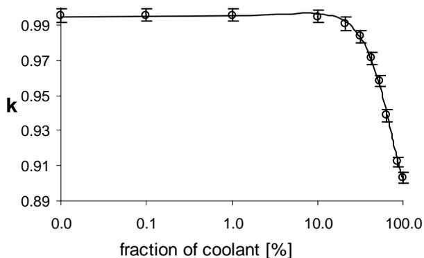
**Fig. 4.** Neutron multiplication factor  $k$  vs. the coolant fraction remaining in the system.
