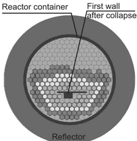
**Fig. 5.** Simplified model of collapse accident.
