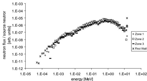
**Fig. 6.** Neutron flux spectra per source particle per lethargy unit in individual zones.
