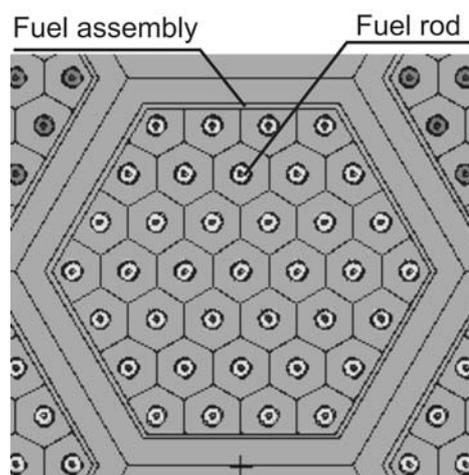
Fig. 2. Fuel element cross section.
