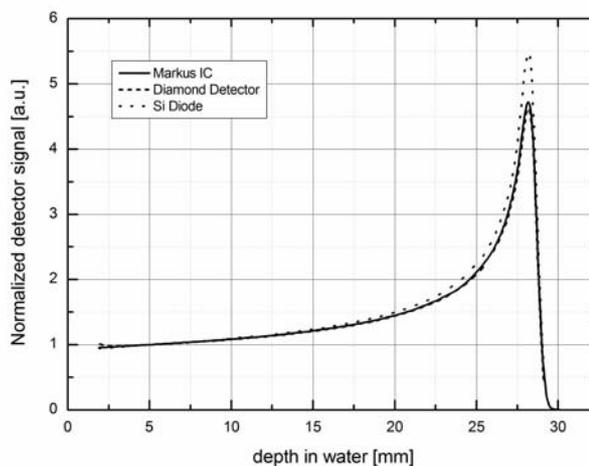
**Fig. 1.** Depth dose curves of proton beam in water measured with Markus IC (solid line), diamond detector (dashed line), Si diode (dot line).
