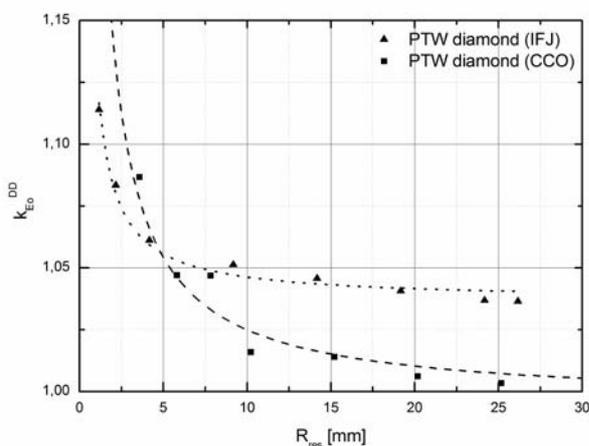
**Fig. 2.** The empirical coefficient  $k^{DD}(R_{\text{residual}})$  for PTW natural diamond detector in the proton beam as a function of residual range,  $R_{\text{residual}}$ , tested in ocular proton beam at IFJ Kraków (values obtained with uncertainty not exceeding 2.5%) and in ocular proton beam at the Clatterbridge Center of Oncology (CCO) [4].
