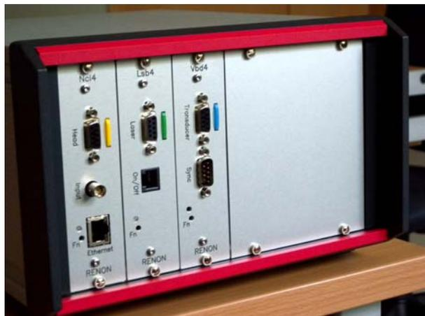
**Fig. 2.** A view of the front panel of the main bin with all the boards inserted, i.e., Ncl4 – nuclear board, Lsb4 – laser calibration board, and Vbd4 – transducer board. A lightning diode on the front panel of each board is an indicator of the operational conditions. The push-button marked as Fn and located close to the lightning diode enables software pre-selected internal functions.
