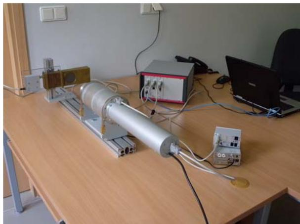
**Fig. 1.** A general view of the complete MsAa-4 spectrometer with a proportional detector head and a Kr-filled proportional counter. The laser high voltage cable is not connected as well as the CAN unit shown. This version is operated directly from mains.
