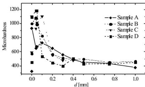
**Fig. 4.** Microhardness distribution in the cross-section of nitrided cast steels ( $d$ -depth under the nitrided surface). Single experimental points represent surface microhardness of as-cast samples. The relative uncertainties are about 5%. Evaluated dispersion originated from inhomogeneity of the material is equal to  $\pm 50$ .
