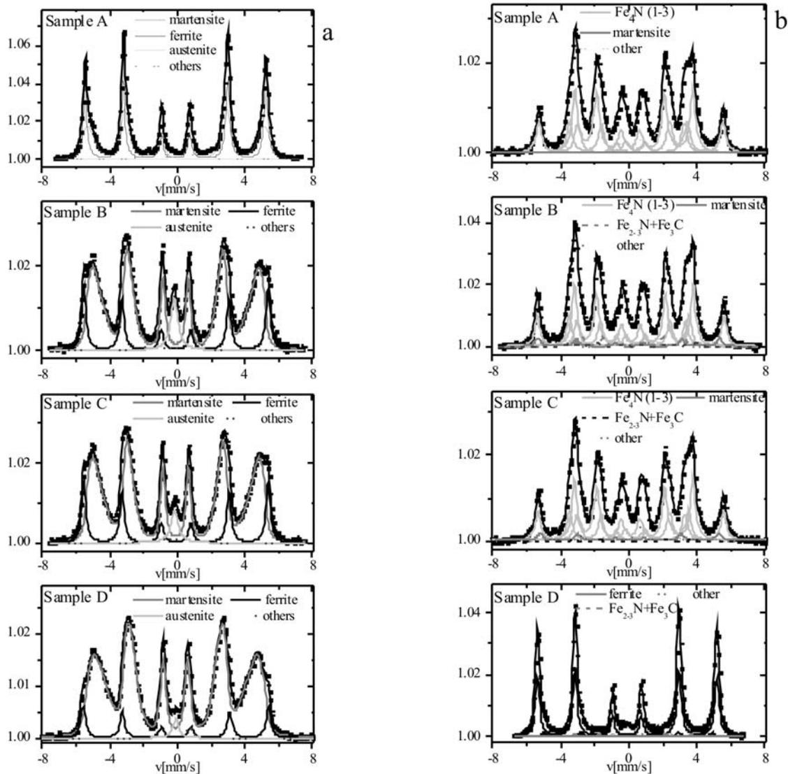
**Fig. 2.** Mössbauer spectra collected for as-cast (a) and nitrided (b) cast steels.
