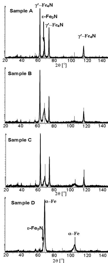
**Fig. 1.** XRD patterns obtained for nitrided cast steels. Some main peaks of identified phases are shown at the pictures.
