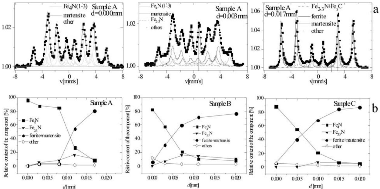
**Fig. 3.** Layer-to-layer analysis: Mössbauer spectra collected for sample A at the depth *d* under the nitrided surface (a) and distribution of iron over individual phases vs. *d* derived from CEMS spectra collected for cast steels A–C (b) (the absolute uncertainties are about 5%).
