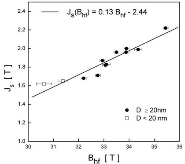
**Fig. 2.** Saturation magnetization vs. HMF induction for mechanosynthesized  $\text{Co}_x\text{Fe}_y\text{Ni}_z$  alloys. The error bars of  $J_s$  do not exceed the area of points plotted on the graph.
