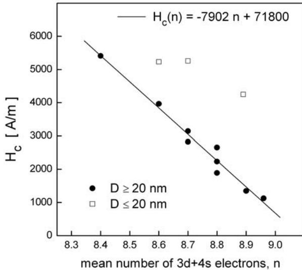
**Fig. 3.** The dependence of coercive field on the mean number of  $3d+4s$  electrons for mechanosynthesized  $\text{Co}_x\text{Fe}_y\text{Ni}_z$  alloys. The error bars of  $H_c$  do not exceed the area of points plotted on the graph.
