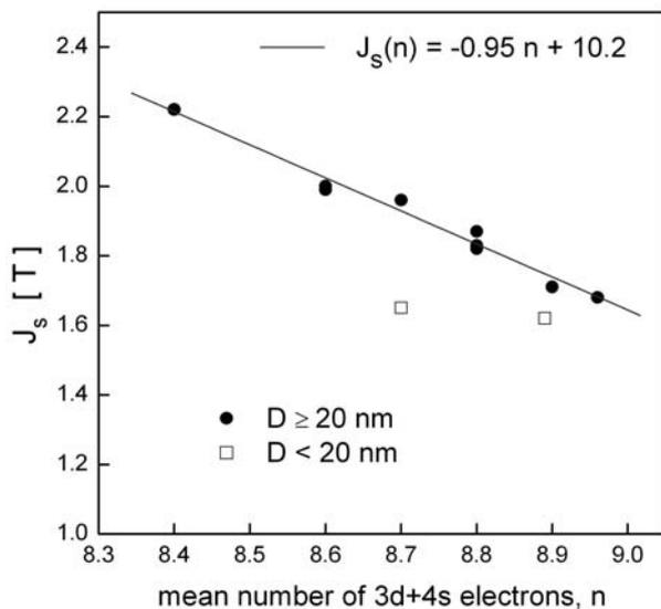
**Fig. 1.** The dependence of saturation magnetization on the mean number of  $3d+4s$  electrons for mechanosynthesized  $\text{Co}_x\text{Fe}_y\text{Ni}_z$  alloys. The error bars of  $J_s$  do not exceed the area of points plotted on the graph.
