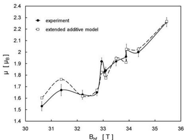
**Fig. 6.** The average magnetic moment vs. HMF induction for mechano-synthesized  $\text{Co}_x\text{Fe}_y\text{Ni}_z$  alloys – comparison of experimental data and the values obtained from the extended additive model.
