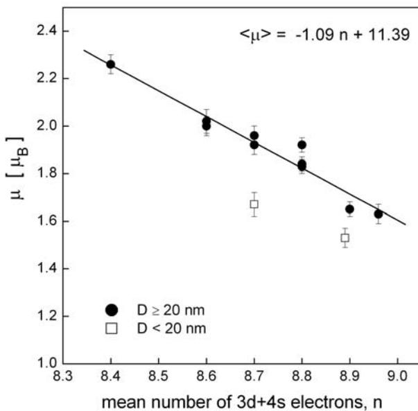
**Fig. 4.** The dependence of average magnetic moment per formula unit on the mean number of  $3d+4s$  electrons for mechanosynthesized  $\text{Co}_x\text{Fe}_y\text{Ni}_z$  alloys.
