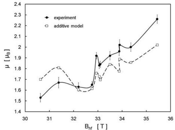
**Fig. 5.** The average magnetic moment vs. HMF induction for mechanosynthesized  $\text{Co}_x\text{Fe}_y\text{Ni}_z$  alloys – comparison of experimental data and the values obtained from the additive model.
