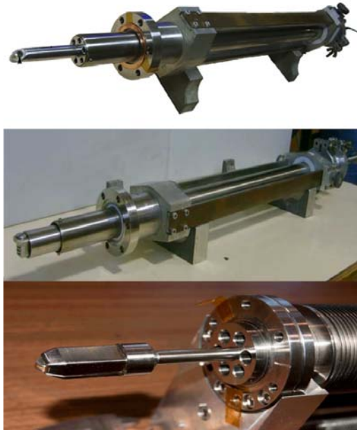
Fig. 2. Different versions of the Cherenkov-type detectors designed especially for fast electron measurements within the ISTTOK tokamak; (top) a single-channel detector with an AlN radiator; (middle) a 4-channel detector with AlN radiators, (bottom) a new single-channel detector with a diamond radiator.
