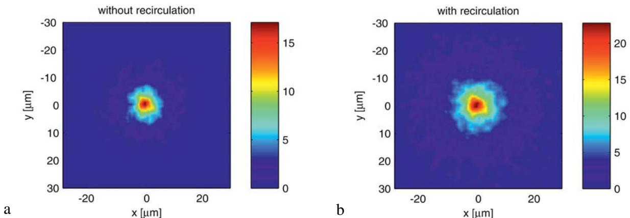
**Fig. 3.** The total count of K- $\alpha$  photons radiated from the rear side of a 10  $\mu\text{m}$  thick copper slab target, per one million initial hot electrons with the Boltzmann–Maxwell distribution corresponding to the temperature of 200 keV per pixel. The size of the pixel is 0.8  $\mu\text{m} \times 0.8 \mu\text{m}$ . (a) The refluxing was not taken into account. (b) The refluxing was taken into account. The colors were smoothed using a convolution mask.
