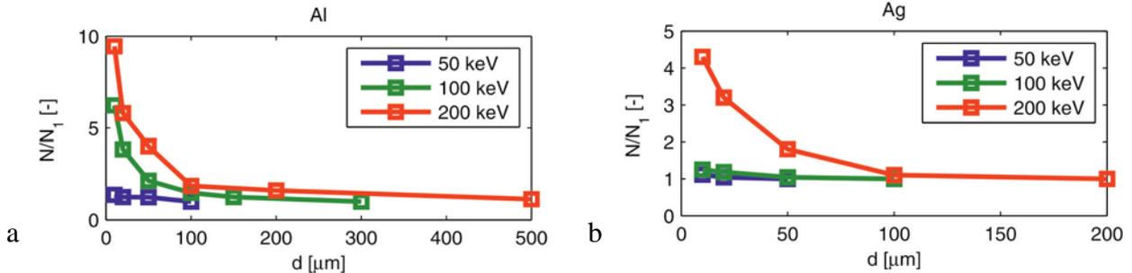
**Fig. 2.** A relative increase in the count of the detected characteristic K- $\alpha$  photons, represented by  $N/N_1$ , when the hot electron refluxing is taken into account, as a function of the width  $d$  of the slab target, for various hot electron temperatures and for two different materials, aluminum (a) and silver (b).
