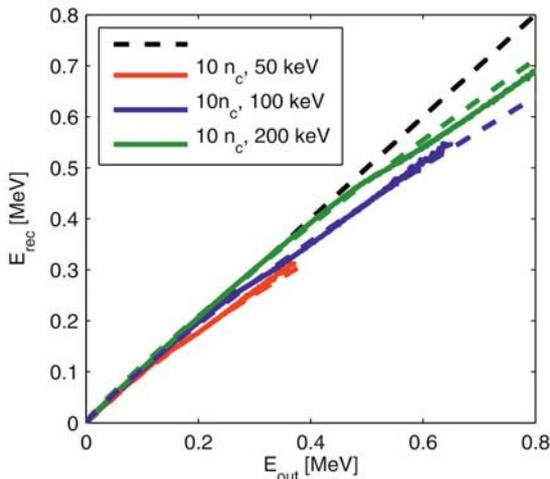
**Fig. 1.** Numerically simulated dependence of the average returning recirculating electron energy on the energy with which they left the target, for different hot electron temperatures. A model expectation according to Eq. (1) is plotted for comparison.
