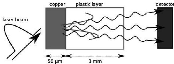
**Fig. 4.** A simple experimental setup designed to demonstrate the effect of the electron refluxing on the K- $\alpha$  radiation.
