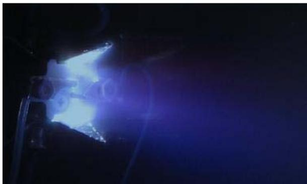
**Fig. 7.** On the top, a photograph of the thruster with a small discharge is presented. The light blue color between the small electrodes indicates the path of the discharge that ionizes the propellant. At the bottom, the main discharge at 900 V is shown, which is responsible for the acceleration and thrust generation.
