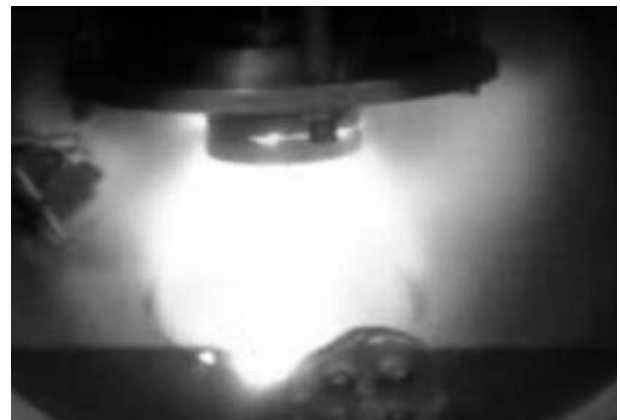
Fig. 2a. Plasma jet in a high-current operation mode. The plume is observed perpendicular to the acceleration direction.
