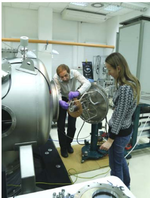
Fig. 2. Vacuum stand for testing plasma thrusters and exposed rear flange.
