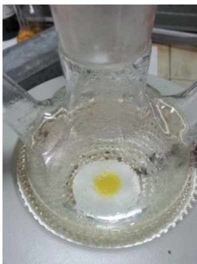
Fig. 8. ‘Yellow cake’ precipitated from acidic pregnant leach solution PLS-3.
