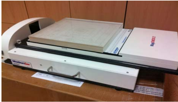
Fig. 2. The robotic platform (MotionSimXY/4D; Sun Nuclear, Melbourne, FL, USA) with diode array (MapCHECK 2; Sun Nuclear, Melbourne, FL, USA) and water equivalent built-up (3 cm of solid water).
