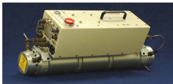
Fig. 2. Thermo Scientific MP 320 portable neutron generator.
