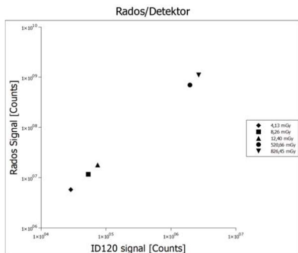
**Fig. 4.** Comparison of the signal intensities obtained with the commercial RADOS device and the tested ID120 semiconductor detector.
