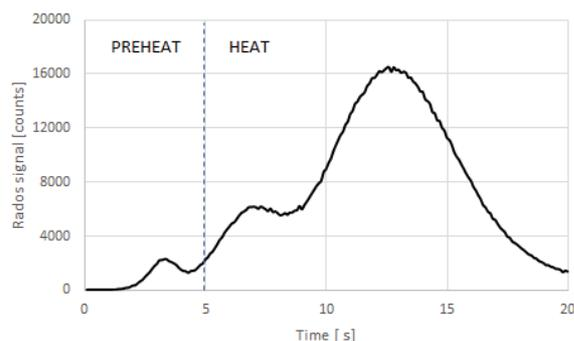
**Fig. 1.** Typical glow curve of the TLD readout obtained with a commercial RADOS detector. Two phases of the measurement, namely, preheat and heat, are indicated.
