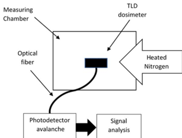
**Fig. 2.** Measurement setup composed of two main blocks – one related to the heating system, and the other responsible for optical system detection and analyses.
