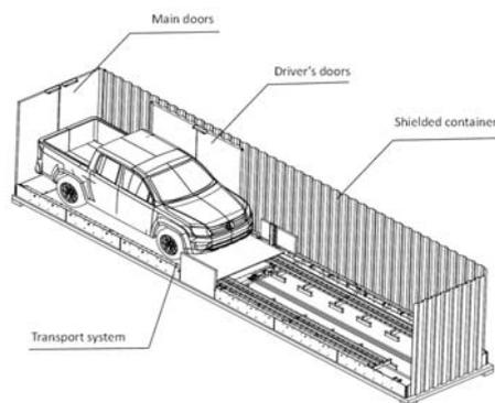
Fig. 3. Main elements of the Sowa scanning system.
