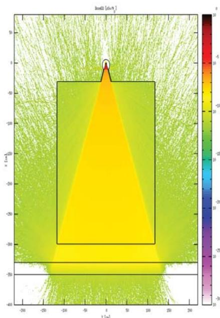
**Fig. 4.** Distribution of the dose rate during the scanning of the container – an example of Monte Carlo simulations.
