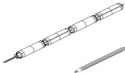
Fig. 5. Top: Isometric view of the instrumented material sample containers. Bottom: Isometric view of the electrical heater coils.
