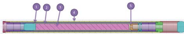
Fig. 8. Geometrical model. 1 – inner shell, 2 – electrical heater, 3 – samples with holder, 4 – outer shell, 5 – “crown”.
