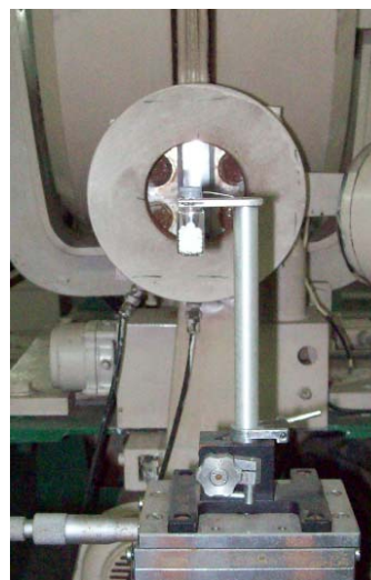
Fig. 2. LAE 13/9 electron accelerator in the setting for direct beam irradiation. Bottle with a PP sample on the background of the accelerator window.
