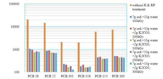
Fig. 5. Comparison of NDL-PCB concentrations in untreated sediment samples with RP-treated samples following HT.
