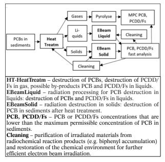
**Fig. 3.** Block diagram of the design of optimization of interconnection of HT methods with radiation treatment method in their complementary interaction.
