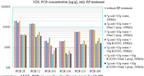
Fig. 4. Concentrations of NDL-PCBs in samples of sediments treated with RP.
