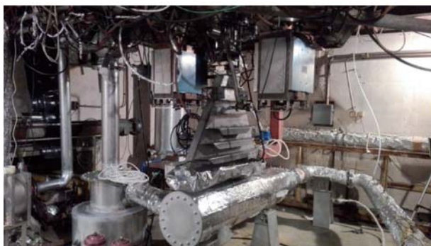
Fig. 4. Photo of EBFGT pilot laboratory flow system. Wet scrubber (left) and process vessel (right) under ILU 6 electron accelerator scanning horn.
