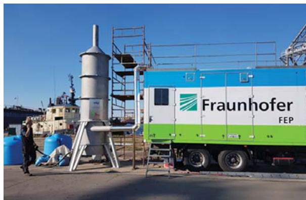
Fig. 7. Photo of EBFGT installation at Riga Shipyard. Mobile accelerator unit (right) and wet scrubber (left).
