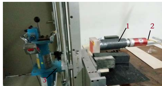
Fig. 1. Experimental setup from left showing the Am-241 in the blue containment shield, the ACR phantom placed in the mechanical arm surrounded with lead blocks to stabilize the arm movement, and finally is the NaI detector with a lead sleeve to shield it from the scattered radiation. 1 – ACR phantom, 2 – NaI crystal, 3 – Am-241 source.
