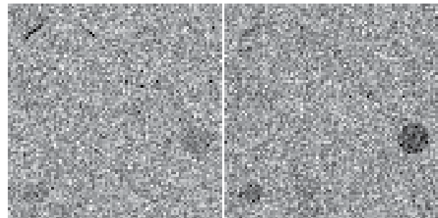
Fig. 6. Images produced with 59.5 keV photons (left) and 26.3 keV photons (right) using 1 mm openings.
