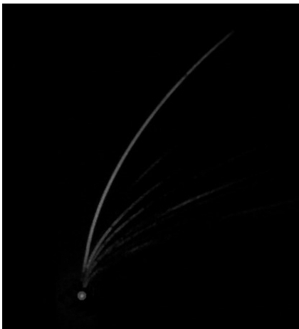
Fig. 1. Parabolas registered on a microchannel plate coupled with a phosphor screen.
