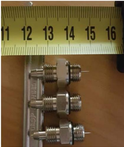
**Fig. 6.** The gas injection system was homemade with 200  $\mu\text{m}$  clinical needles glued (epoxy) in the gas rail couplings.
