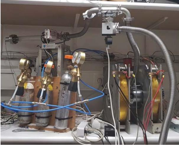
**Fig. 5.** Common rail vacuum system serves both experiments. On the left is the Langmuir probe and on the right is the EM cavity each with its own injection system but sharing the same gas rail. Only the EM cavity is equipped with magnetic field coils.
