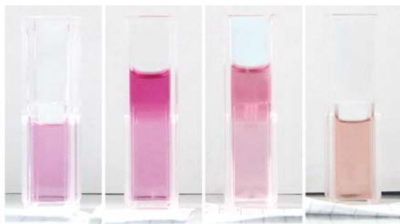
**Fig. 5.** Roselle dosimeter irradiated at 0, 0.6, 1.3, and 2.5 kGy.
